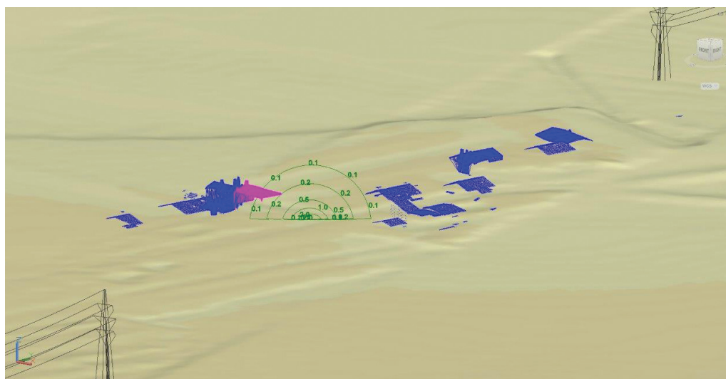
Figure 15: Presentation of a detailed micro location calculation of the magnetic field B [ \mu\text{T} ] on a perpendicular plane to the underground cable axis at the selected object.
