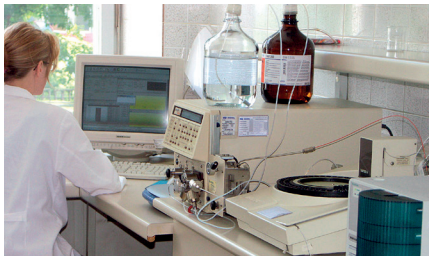
HPLC Furanic analyses for evaluation of paper insulation ageing
