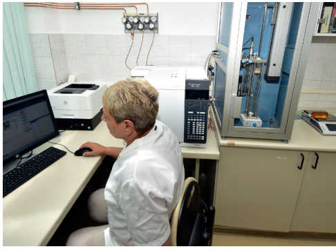
Detection of electrical and thermal faults of operating transformers by DGA gas chromatography with vacuum extraction
